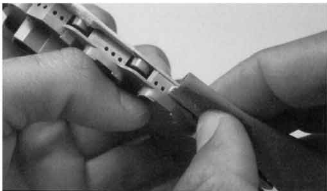
Seam lines that run across porthole detail are not hard to fix, but it takes a little time. Wrapping sandpaper around a piece of balsa wood fixed this problem on Revell's 1/426 scale Arizona .
