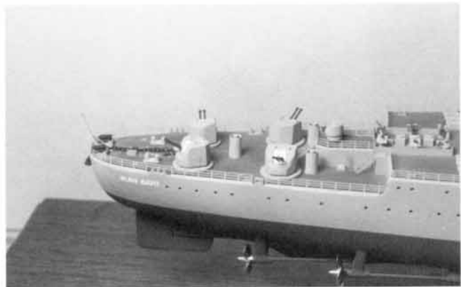
Railings can stop and start at deck fittings, or you can cut stanchions out of a length of railing so that you have a continuous length.
