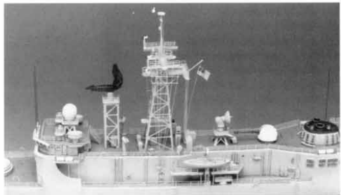
The railing lengths on the upper deck of this resin model were done in sections because of the numerous small bends and curves along the deck line. Model by Lonnie Ottzen, master pattern designed by John Ficklen, photo by Glenn Johnson.
