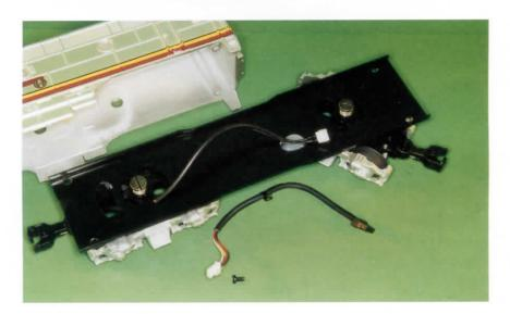
Now the B-unit looks better. We stored the wire and screw in a zip-lock bag and put the bag inside the B-unit's box so that we can reinstall it later.
