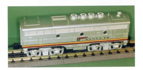
Simple modifications and maintenance will keep your MTH trains running for a lifetime. The B-unit for the F3 locomotive set has an external wire for the optional digital sound system. Since our locomotive has only a horn, we removed the external wire.
