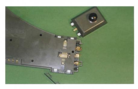
Here you can see the clean and simple design of the underside of the switches. There are no wires or screws to mess with, and here again, MTH designed their switches to be plug-and-play.
