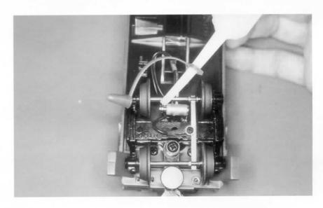
One last tip on lubricating is to add a drop of oil to the axles of the pickup rollers of lighted freight and passenger cars.
