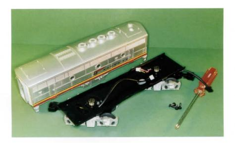
Next, we removed the wiring harness screw from the truck and pulled out the wire.
