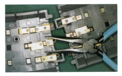
The simple fix is to use a set of needle-nose pliers to bend the brass contact back into shape.
