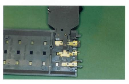
Here you can see the positive brass connectors designed to ensure that any device or accessory plugged into the track system will not experience voltage drop due to poor electrical contact. MTH has a complete line of sturdy die-cast accessories from which to choose. Two favorites are the operating block signal and the crossing gate.
