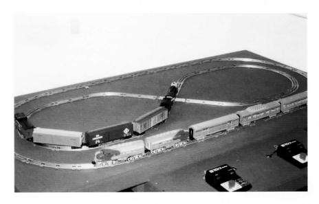
This is how standard track looks on a train board. To deaden the sound of the trains and to improve the appearance of the track, roadbed is placed under the track, additional ties are inserted under the rails, and scale gravel is spread over the cork roadbed.
