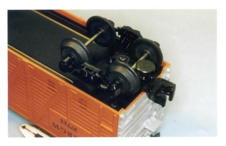
The disks located on the bottoms of the couplers are for uncoupling. When the disk is located over an uncoupler track and the uncoupler is activated, the disk is drawn down, which opens the coupler.
