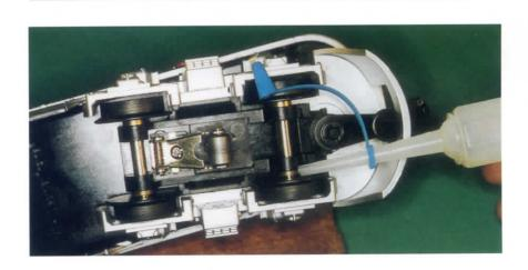
Diesel locomotive axles should be lubricated so the contact points between the wheel ends and the trucks will not wear out. While you should purchase train-lubricating oil, a light sewing-machine oil will do. Lubricating the gears is an absolute must for all diesel locomotives. Small quantities applied to each gear work best.
