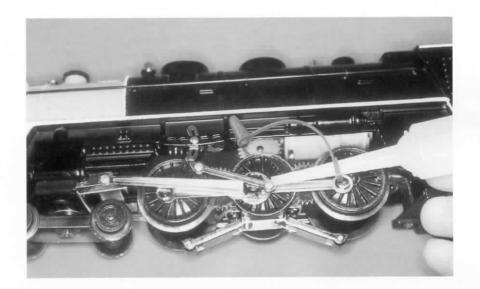
When lubricating the gears on a steam locomotive, do not forget to lubricate the bearings of the running gear and the drive rods.
