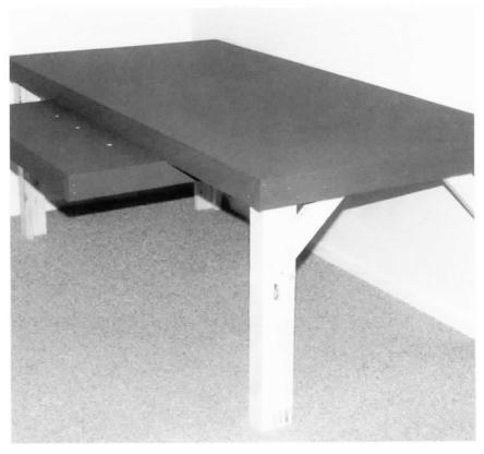
The control panel and train board surfaces have been painted dark green, and we're now ready to lay out track and run some trains. The construction techniques used to build this train board are very simple, yet the board is so strong and stable that you can stand on it.
