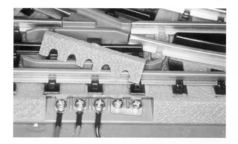
Here the wire bundle ends are attached to the screw posts on the switch. Be sure that the brass jumper (at right) is not removed, as this is the internal jumper that tells the tiny motor inside the turnout to get its power from the track instead of an external source.
