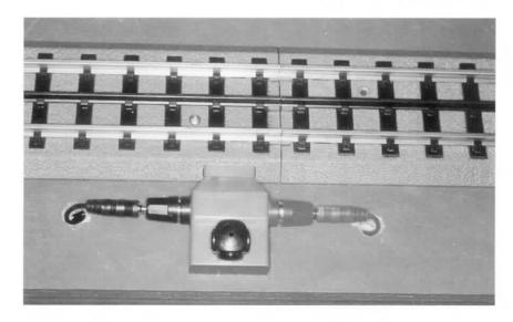
Note how the lock-on wires are connected. There is no excess wire on top of the plywood.
