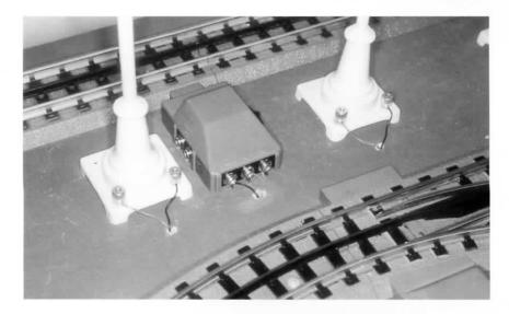
This infrared sensor has a three-wire hookup to the block signal for the siding. Accessory hookups will use the common screw post and either or both of the "NC" and "NO" screw posts.
