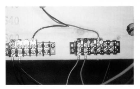
Position terminal strips in a location under the train board so you can minimize the lengths of wire bundles from the terminal strips to the structures. The upper two wires go back to the switch on the control panel. The terminal jumper distributes power to all the screws it is attached to, and the lower wires come from the individual structures.
