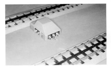
Next, I plugged in the infrared sensors at the far ends of the track so that the crossing gate signals would be activated by a train approaching from either direction. The crossing gate signal is a simple two-wire hookup to the common and "NO" screw terminals of the sensor.
