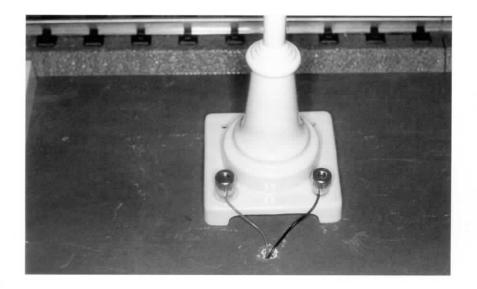
These die-cast metal lights are easy to hook up. I used telephone wire for these applications because it's inexpensive, and the wire is solid which means that you can shape it. Radio Shack sells lengths of this telephone wire, which has four colored wires: red, black, yellow, and green. In most applications I simply use two wires—red (hot) and black (ground).
