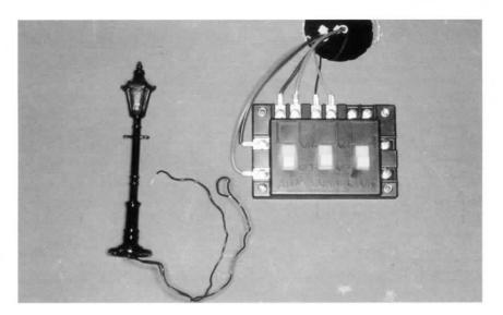
The wires attached to these small lamps are also stripped. I tested the lights by touching the wires to the screw posts on the left side of the Atlas connector.
