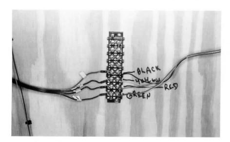
Next, I attached the colored wires to the corresponding screw post on the uncoupler.
