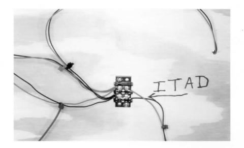
Since the infrared sensors draw their power from the track, there is no need to add an additional power source. You can even hook these sensors together so that you can activate an accessory from separate locations. Here two wires come from each sensor and from each crossing gate signal. To keep from mixing up the polarity of the sensors and the accessories, I used red and black wire.
