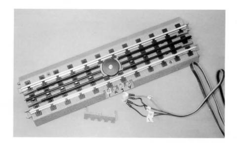
I positioned a terminal strip under the train board and then attached the labeled wires. Then I attached the telephone wire to the terminal strip and labeled each color (which I then wrote down) so that each label (1 through 4) had a corresponding colored wire.
