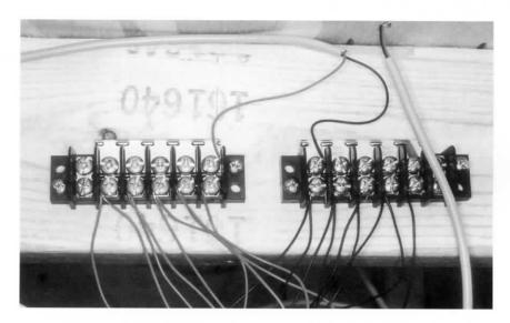
Since I planned to have all the die-cast streetlights controlled by one of the Atlas connector switches, I added these wires to the yard light terminal strips.
