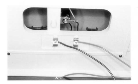
All of the ready-built structures have simple wire clips to hook into. Strip about 1/6 inch off the ends of the wire, twist it (if it's stranded), push the clip back, and insert the wire.
