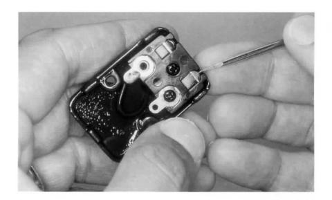
Here the wires have been attached. Note that the insulation on the wire has been removed only far enough to attach to the clip.
