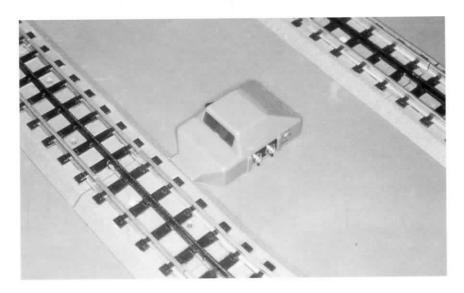
The two infrared beams emit from the red plate of the sensor, so it's important to protect the surface of this plate. You can adjust the range of the sensor from as close as 1½ inches to as far away as about 14 inches.
