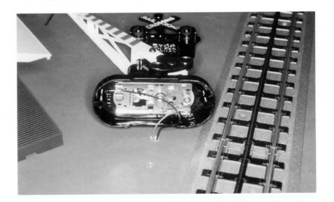
The crossing gate signals had quick-attachment wire clips that make wiring them quick and easy.
