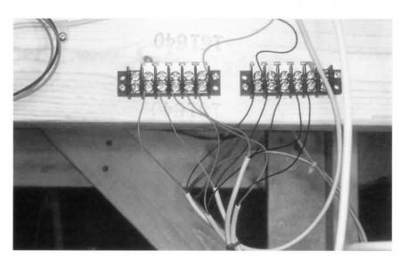
The die-cast yard lights have all been connected to the terminal strips, and power from the Atlas connector has also been attached. I used the second switch on the Atlas connector for the die-cast lights. Notice how the tie strips help keep wire bundles together as well as minimize the messy appearance of large quantities of wires. One last thing to do is flip the switch and test the lights.
