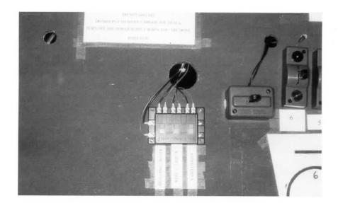
To help us with all the switch locations, I labeled the switch controllers and also added a simple layout diagram with the corresponding labels on the switches.
