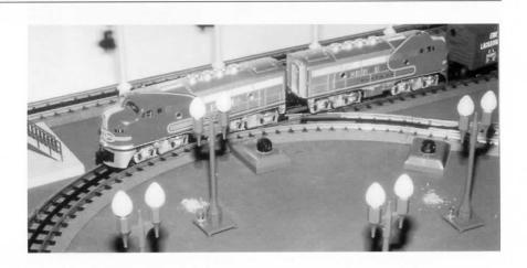
The screw posts on some of the die-cast lights have holes in them, which makes attaching the wires very easy. Also note that one terminal post is insulated from the rest of the accessory.
