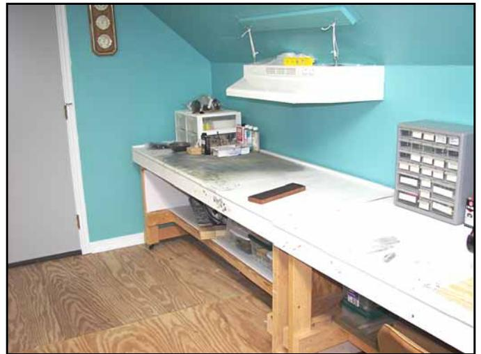
My airbrush station discharges outside the room. All I need to do is add foam board sides to box off the area under the vent hood to concentrate the air flow.
