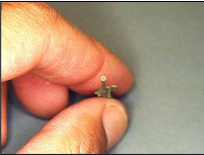
To hollow out the tip of the 50 caliber machine gun I indented the surface close to the center to help set the tip of the drill bit.
