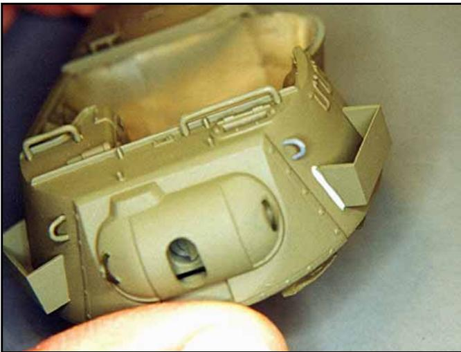
The storage bin sides did not fit correctly onto the curved surface of the turret. I applied a tiny bead of white glue along the void with a small diameter wire applicator.
