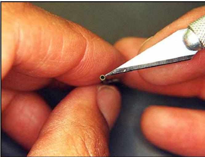
I finished the opening by peeling away a few layers of plastic with the tip of a sharp number 11 X-Acto blade.
