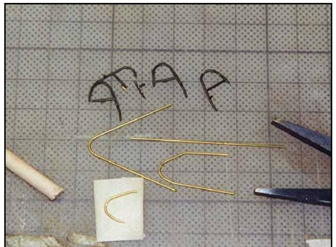
The kit supplied brush guards were not well molded so I made new ones with thin diameter stiff brass wire. I shaped the curves with a wood dowel.
