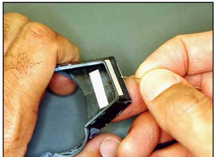
Once the tracks were completed I turned my attention to the turret. I taped the turret halves together and then applied a bead of super glue along the seam line.
