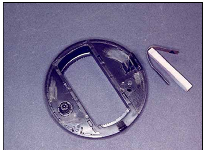
I carefully sand off the injection pin marks on the base of the gun mount using various grits of sandpaper wrapped around a small length of balsa wood.
