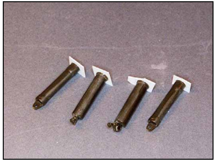
To reduce the size of the openings I laminated .015 inch sheet stock onto the face of each part.
