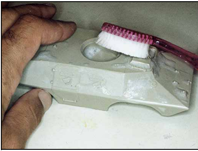
The first step in working with resin parts is to wash them to remove any mold release agents that may still coat the parts.
