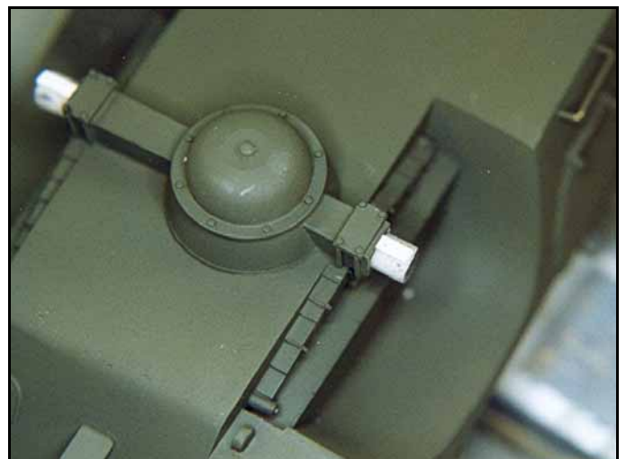
The wheels openings for the axles were larger than the axle diameters so I added small bits of plastic to the axles to make up the difference.
