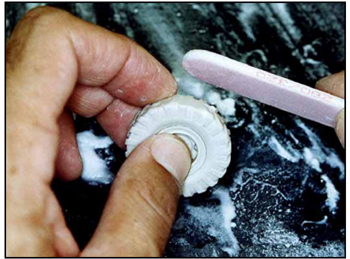
To remove the remaining pour plugs on large parts wet sand the resin off with a sanding stick.
