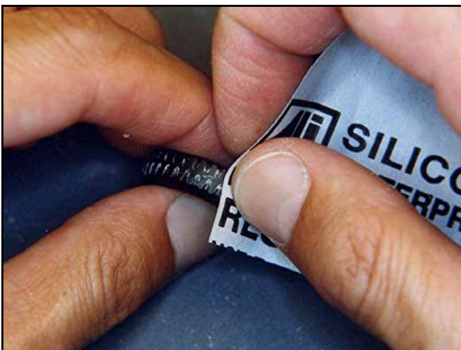
Next carefully smooth out the seam line by wet sanding using water proof sandpaper.
