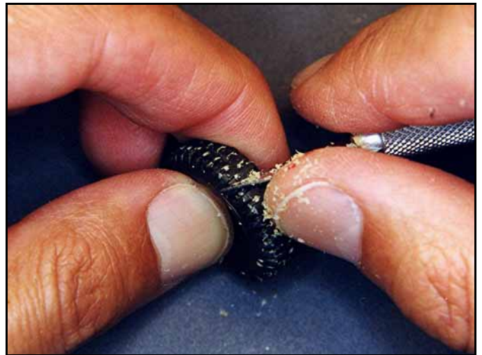
Once the glue is dried carefully scrape the surface of the seam to remove any excess super glue.
