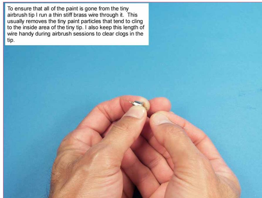
To ensure that all of the paint is gone from the tiny airbrush tip I run a thin stiff brass wire through it. This usually removes the tiny paint particles that tend to cling to the inside area of the tiny tip. I also keep this length of wire handy during airbrush sessions to clear clogs in the tip.
