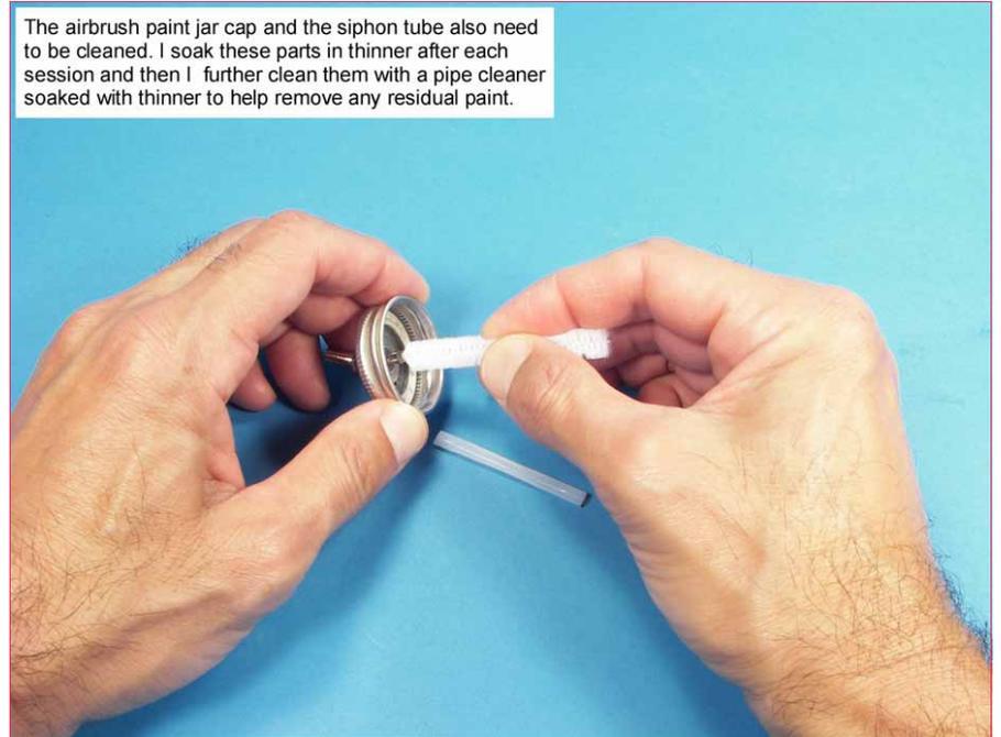
Your airbrush should be taken apart after each painting session and the parts soaked in thinner. The individual parts will need to be cleaned, dried and then the airbrush can be reassembled.
