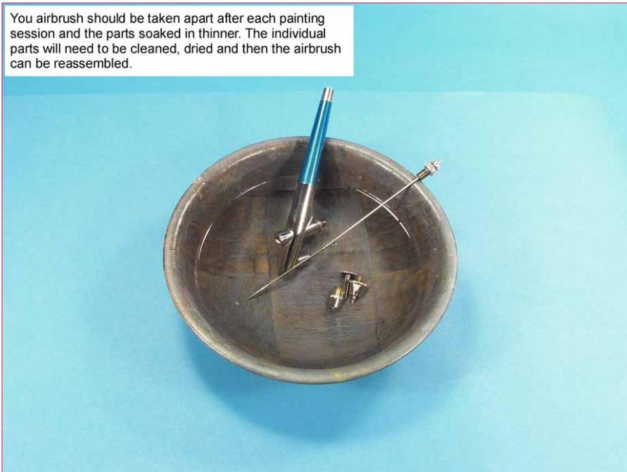
About every six months I remove the two teflon washers from my airbrush and replace them with new ones. In addition I keep a small supply of new tips and needles on hand as they tend to wear out over time. This Badger 200 airbrush has lasted me almost 15 years.
