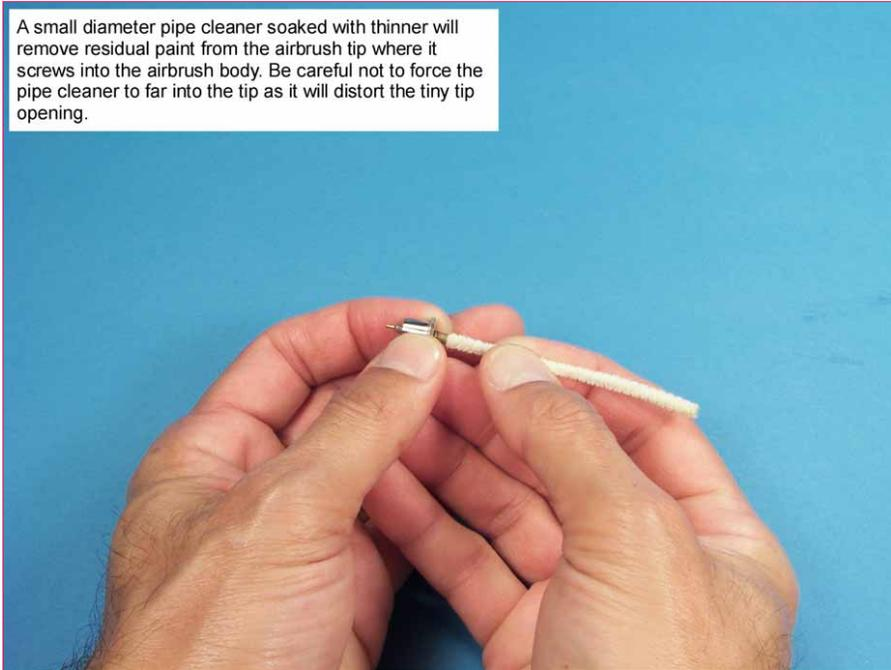
The airbrush paint jar cap and the siphon tube also need to be cleaned. I soak these parts in thinner after each session and then I further clean them with a pipe cleaner soaked with thinner to help remove any residual paint.
