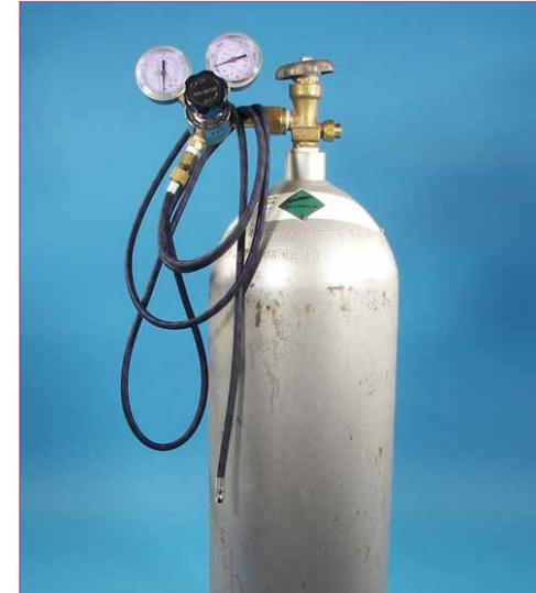
My air source for airbrushing is a CO2 tank with a pressure regulator. The regulator allows me to adjust the air pressure between 1 and 100. The air is always dry and its very quiet. This tank can last up to 2 years.
