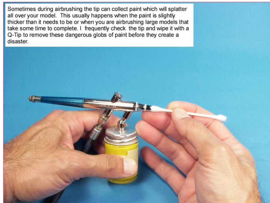
Sometimes during airbrushing the tip can collect paint which will splatter all over your model. This usually happens when the paint is slightly thicker than it needs to be or when you are airbrushing large models that take some time to complete. I frequently check the tip and wipe it with a Q-Tip to remove these dangerous globs of paint before they create a disaster.
