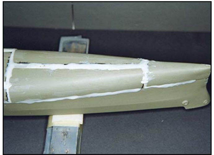
To help fill any remaining gaps between the upper and lower hull I added tiny amounts of resin. One of the great qualities of resin is that new resin sticks to old resin which makes it a great filler!
