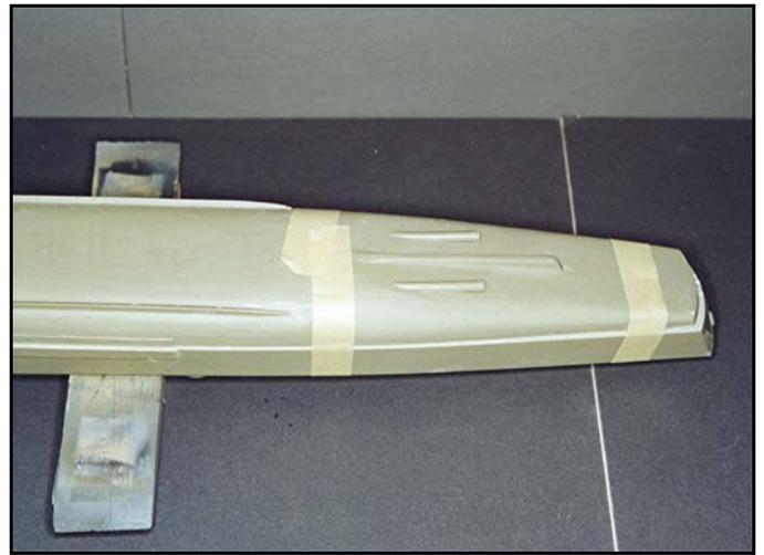
This is a good example of the shrinkage that can occur on resin hull halves. There is no way these parts can be mated together.
