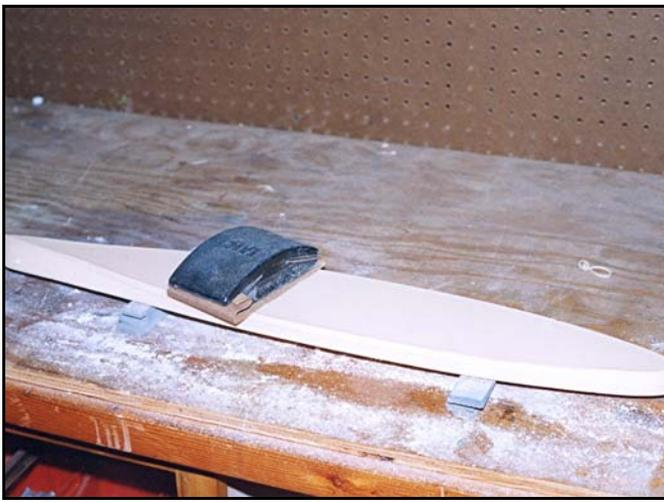
The first step in attaching the upper and lower hulls is to remove any excess casting material. If you do not wet sand be sure to wear a dust mask as the resin particles can irritate your lungs.
