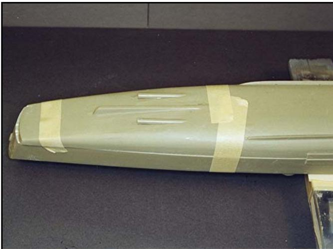
Here is the opposite side of the hull and while the edges are almost lined up there is also a shrinkage problem with the length of the part as well as its width.
