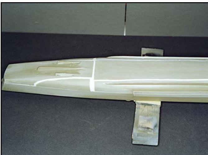
The hull is now almost complete. Once it is primed a final check will be made to fill any remaining imperfections and voids.
