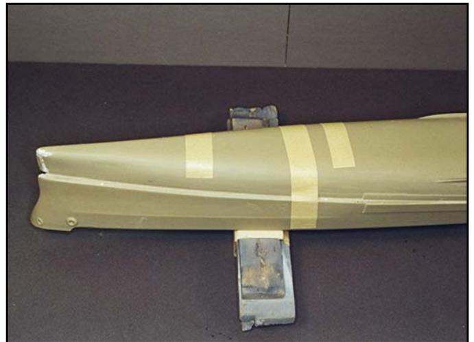
If the shrinkage wasn't enough of a challenge, the lower hull also warped towards the bow!
